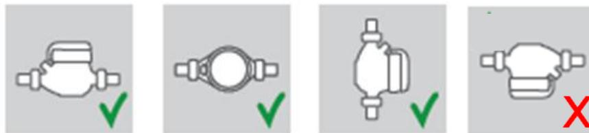
The meters are pre-calibrated and can be mounted in any position (vertical and horizontal) **except** upside down. The design allows for a low risk of corrosion or sedimentation.
