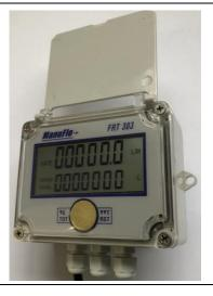
The *FRT303* Flowrate Totalizer is designed to operate with a wide range of pulse/signal output or coil output flowmeters, providing an instantaneous flowrate reading with a resettable Total display and Grand Total display. To toggle the display between the Total and the Grand Total, simply touch the front panel button once. To reset the Total, touch the front panel button twice.
