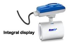
The **KMS501W** electromagnetic flowmeter is capable of operating over a very wide flowrange. It offers reference meter quality performance with accuracy of  $\pm$  0.5% of reading, being ideal for measurement of water and wastewater applications. With no moving parts and an obstruction-less bore, this type of flowmeter guarantees the highest level of performance, whilst maintaining a high degree of accuracy.
