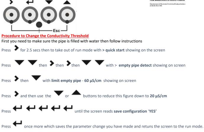
This completes the procedure to Reduce the Change the conductivity threshold. (P.W.King 03/21)
