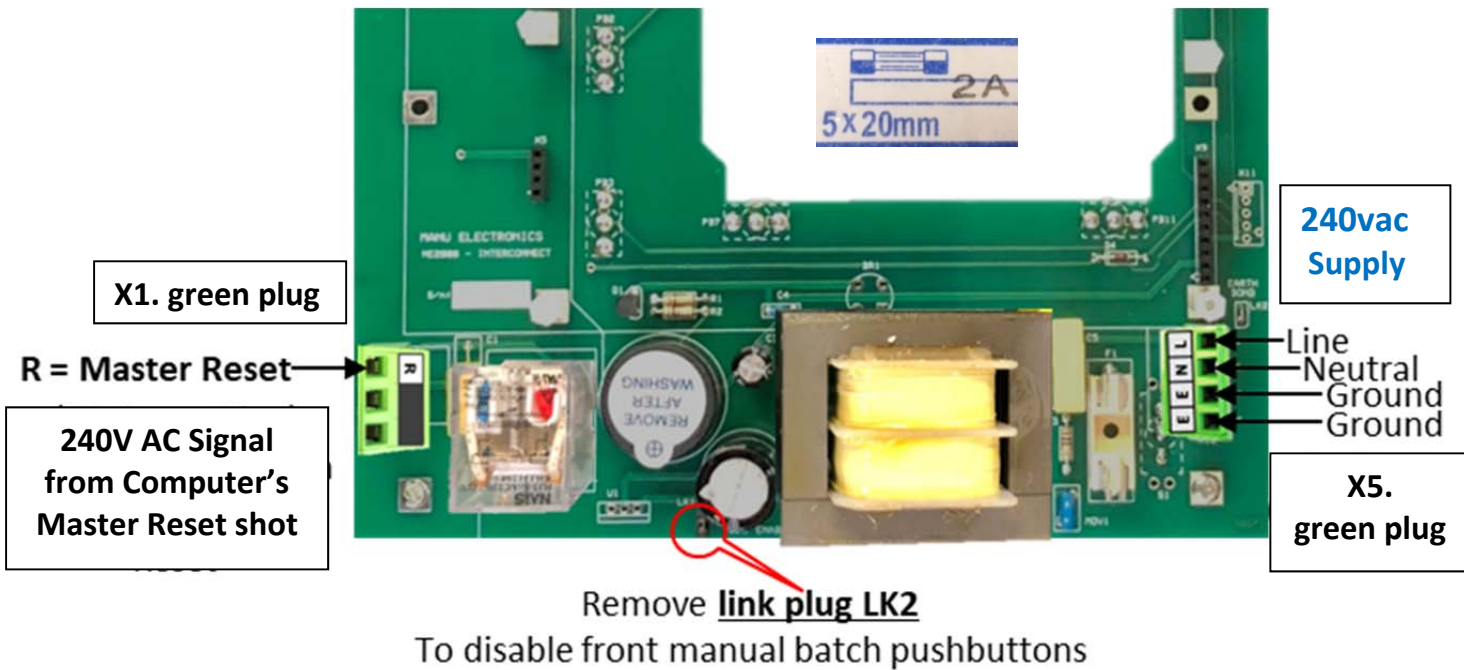
Figure 3. Motherboard Wiring Diagram, X1 and X5 plugs
