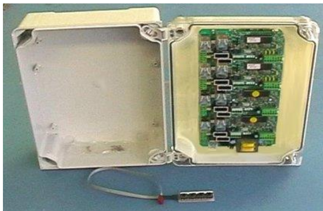
ME2008 8-channel unit, opened, with HP plug-in Programmer.
