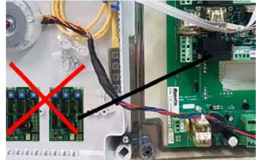
UIC cards wired with internally from ME2008 DC power is not recommended
