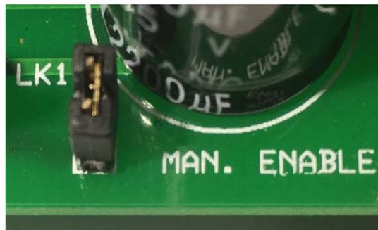
To disable the front manual batch push buttons, remove (with pliers) link (jumper) LK1 located on motherboard near the Alarm buzzer & Capacitor rear bottom of PCB. This will avoid misuse of manual starts. Plug-in LK1 to re-activate manual batch functions.
