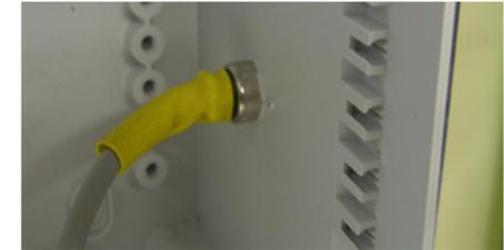
Using the socket as a template, drill two 1/32" holes on either side of the hole, and then use two 1/4" self tapping screws to affix the socket to the ME2008.
