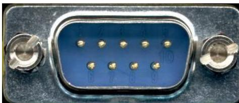
Figure 18. DB9 (Male) Serial connector
