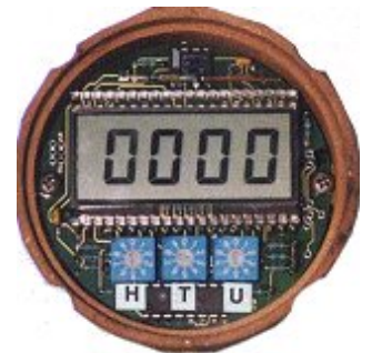
Internal view of calibration HTU switches
