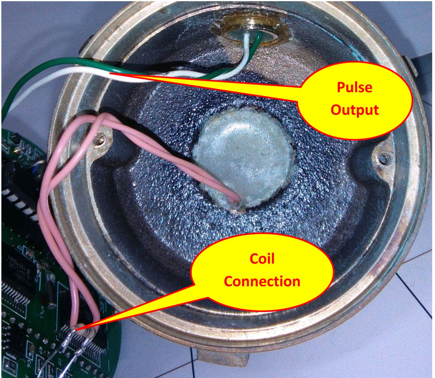
2. Solder the 2pin (Female) connectors provided on both sets of wires coming from the *Coil* and *Pulse output*.
