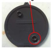
MRT LCD Locked on 'CAL' message likely caused by moisture ingress
