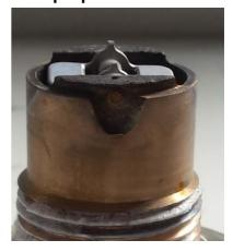
Paddle wheel has been dislodged from mounting position due to a broken axle
