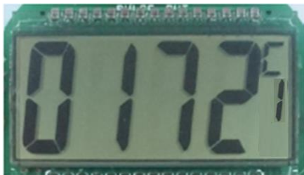
Flowmeter Display once water flow has stopped 'C1' is indicated And numbers shown is Counts/Litre or (Gear Rate/K-FACTOR).
