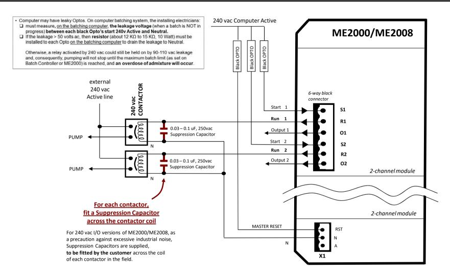
Fitting Suppression Capacitors to prevent electrical noise, and Resistors to prevent voltage leak
