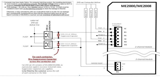
Fitting Suppression Capacitors to prevent electrical noise, and Resistors to prevent voltage leaka
