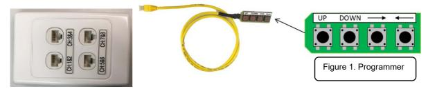
Each Dual Channel Module (DCM) is programmed one at a time. Plug the Programmer into the DCM to be programmed (the programming plug location is shown in
