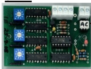
UIC/A1 • switches 110240vac, 512 VDC powered
