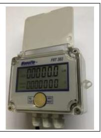
The *FRT303* Flowrate Totalizer is designed to operate with a wide range of pulse/signal output or coil output flowmeters, providing an instantaneous flowrate reading with a resettable Total display and Grand Total display. To toggle the display between the Total and the Grand Total, simply touch the front panel button once. To reset the Total, touch the front panel button twice.
