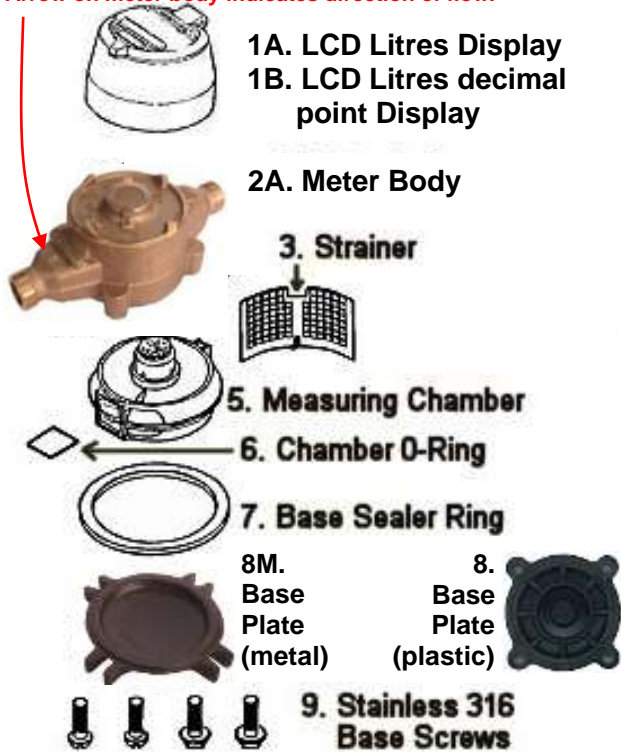
20, 25 & 32mm meter components
