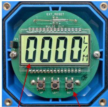
4 digit rate display 3 x calibration buttons
