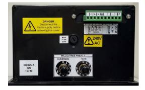
ME995-1 Batch Controller, 240 vac supply and output, with 12 VDC power to flowmeter (standard).
